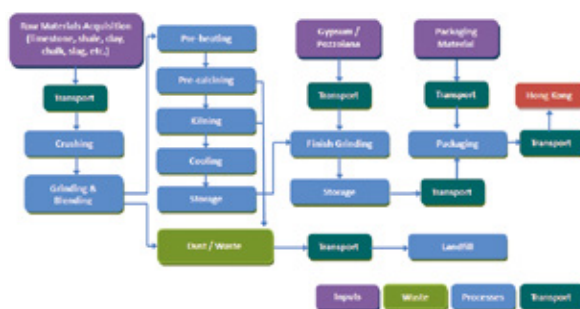
Figure 4. Process Map of Portland Cement Manufacturing 4
