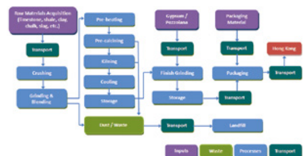
Figure 4. Process Map of Portland Cement Manufacturing 1
