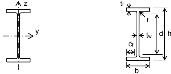
Design Table 01A Section dimensions of rolled I-sections (1)
