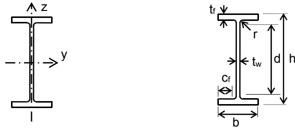
Design Table 14 Section resistances of rolled I-sections: S355 steel (2)
