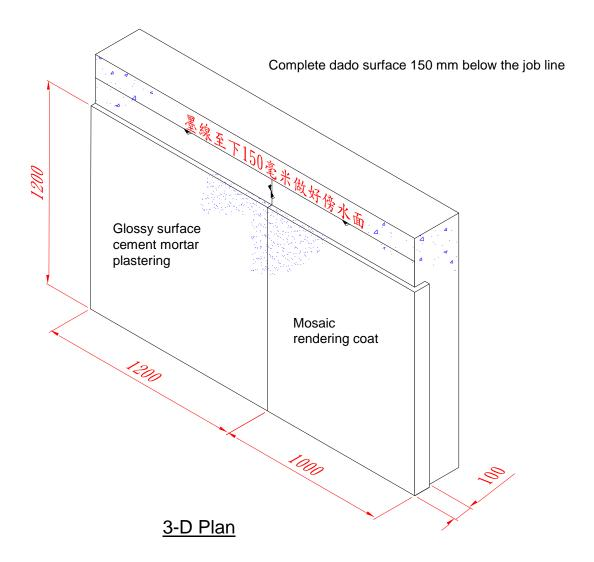
Thickness of second layer of plaster is 8-10 mm
