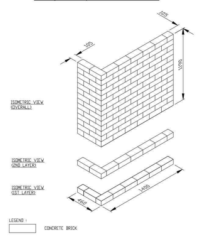
Work elements shown on this drawing are indicative only, please refer to the test paper and onsite test location for details.
