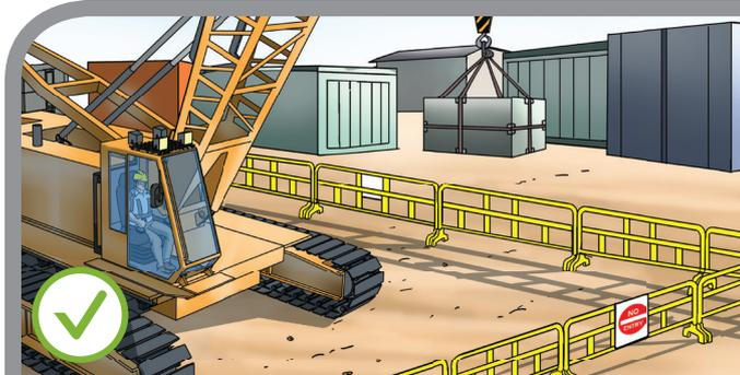
Properly fence the lifting zone with barricades and demarcate with prominent notices and ensure no persons (other than the crane operator) stay within the zone during the lifting operation.
