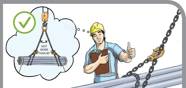
Ensure the safe working load of any multiple sling leg is not exceeded as a result of the angle between the multiple sling legs. Their upper ends shall be connected by means of a shackle, ring or link of adequate strength.
