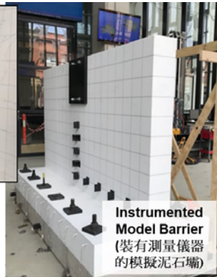
Testing of Boulder Impact (大石撞擊試驗)
