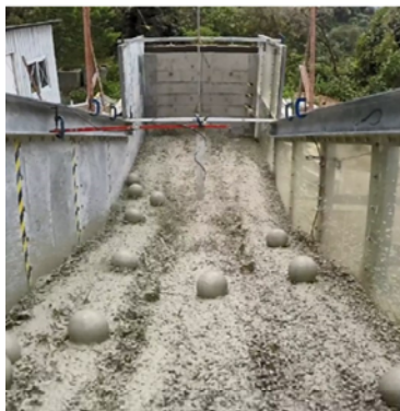
Testing of Debris Impact (泥石流撞擊試驗)
