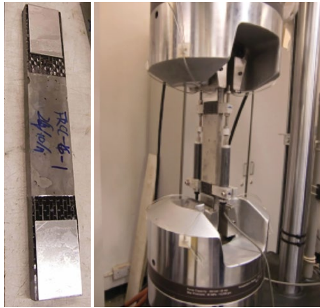
Figure 7 Experimental set up of direct tensile test
