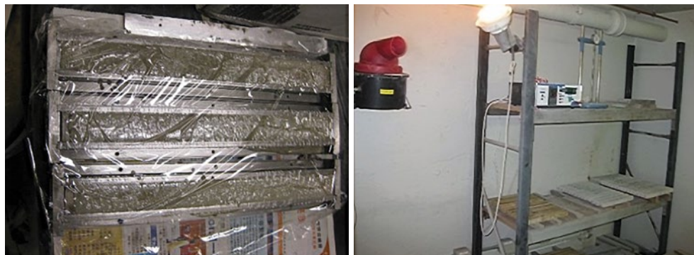
(a) Samples for dry shrinkage test
