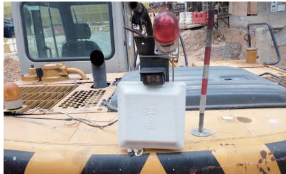
Unsafe Acts / Dangerous Situation Alert System for Mobile Plant Operation Danger Zone
