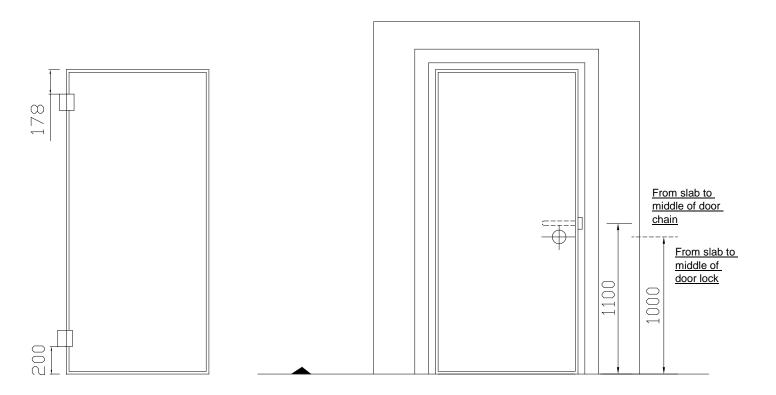
Skills requirement : No assessment on ground clearance of door crack Other 3 sides 2mm from door frame Directions of the door hinges should align with the ground job lines
