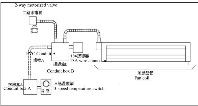
Installation drawing of power system for fan coil (Fig.1)
