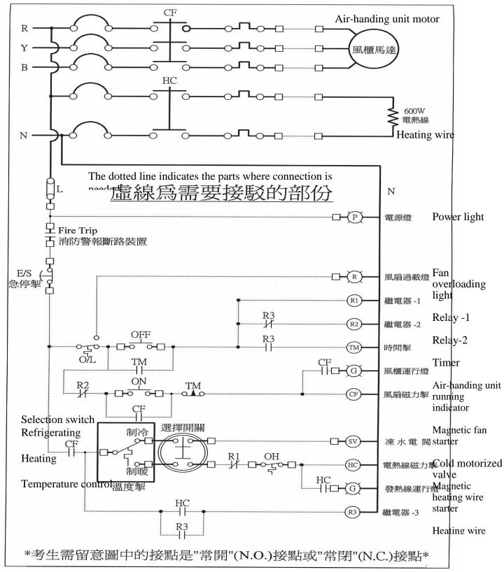
\*Candidates should be aware of whether the contact points in the diagram are "Normally Open" (N.O.) or "Normally Closed" (N.C.) contact points\*
