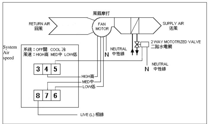
Electricity wiring diagram of 3-speed temperature control (Fig.2)
