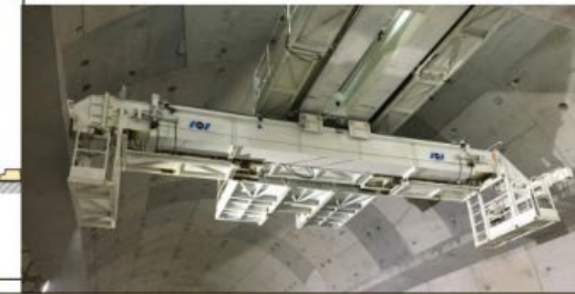
Cross beams telescopically extendable for different Tunnel diameter
