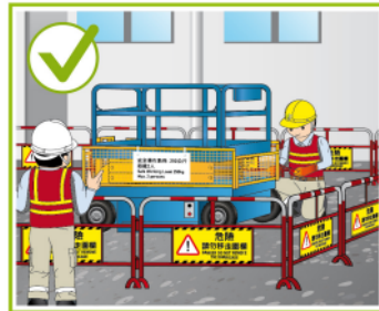
EWP must be parked on a flat ground and the work area must be fenced off for inspection or maintenance work
