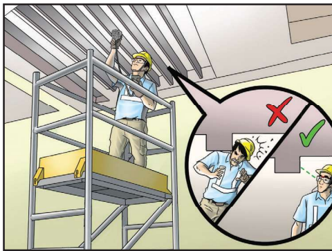
Workers should beware of overhead room and check for any obstruction to prevent accidental hit on the head before and during the use of working platforms. Safety helmets with chin straps should be used.
