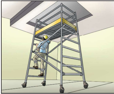
Ascending/descending the mobile working platform from the inside of a mobile working platform.
