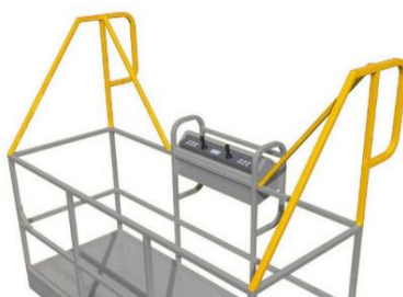
Figure 2: Secondary Guarding Device – Physical Barriers
