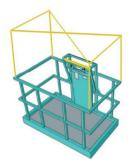
Figure 1: Secondary Guarding Device – Physical Barriers
