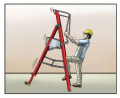
Do not apply excessive force to the working platform and induce lateral force rendering the overturning of the working platform.
