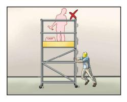
When moving the mobile working platform, no person should be allowed to stand and no object should be placed on the mobile working platform.
