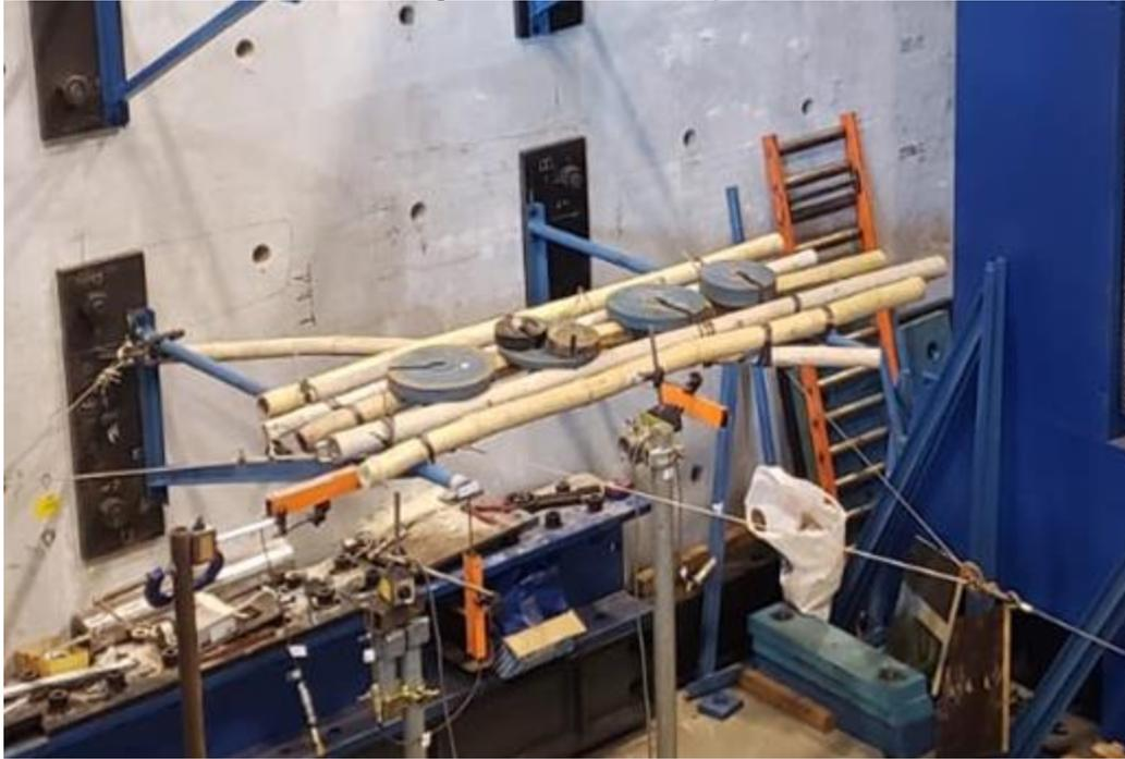
Figure 2 Gravity load test set-up (Uniformly Distributed Load, UDL)
