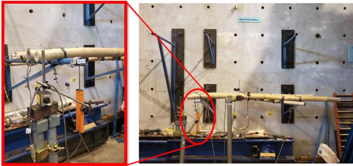
a) Typical test set-up with LVDT for digital deformation measurement
